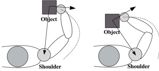
**Figure 1:** Trajectory adaptation through CS transformation. Left: the trajectory is recorded w.r.t. an object-shoulder CS. Right: for playback, an updated object-shoulder CS is constructed, yielding a rotated and scaled trajectory.
